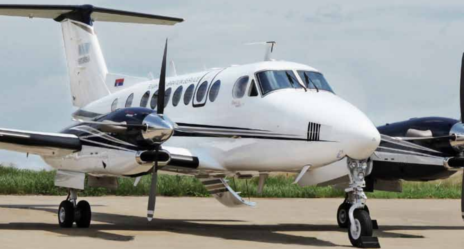
Figure 14: Aircraft for Flight Calibration of Ground NAV Aids - Hawker Beechcraft King Air 350
