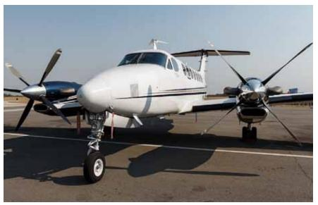
Figure 4. Aircraft for Ground-Based Radio Navigation Aids Flight Calibration – Hawker Beechcraft King Air 350
